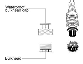
**4.** Rotate the knurled retaining ring until snug on the housing bulkhead. Do not use pliers or tools to tighten the retaining ring.
