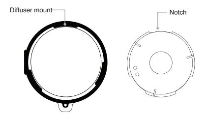
3. Press the diffuser down and rotate counter-clockwise until it stops.
